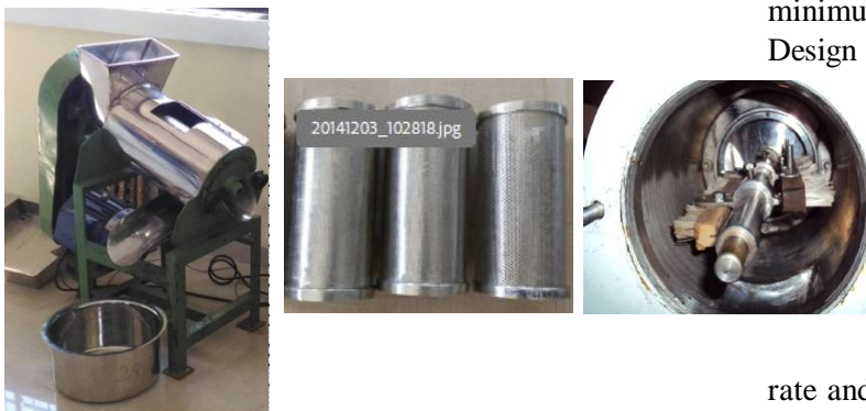
Fig. 1 : Pulper with sieve and brush arrangements.
